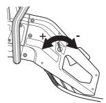
Ample water flow is needed for maximal blade life.
