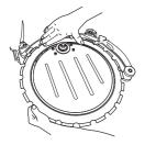
Fit the support roller guard and ensure that the flanges on the guide rollers still enter the blade's grooves correctly.
